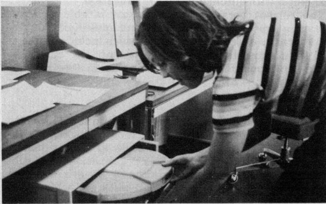
Figure 4. Inserting the disk pack in the Dynabook.
